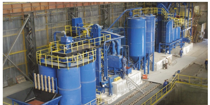
Installation of enveloped sands lines Q=4 t/h
