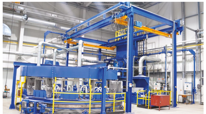
Box moulding lines - VACUUM PROCESS technology
