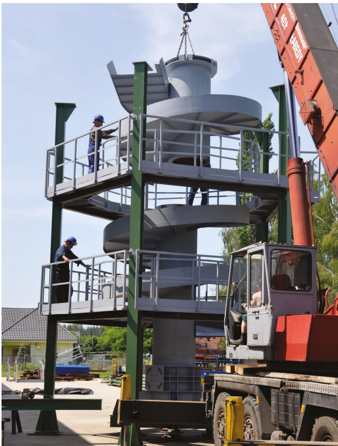
Vibrating vertical conveyors for transporting castings
